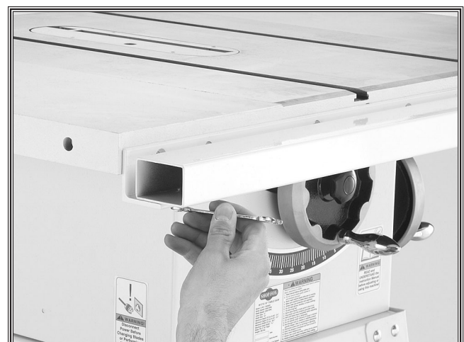
Figure 4. Installing fence tubing.
